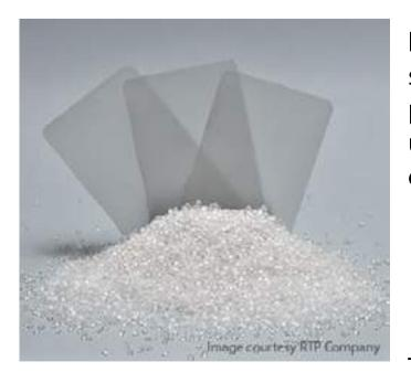
I needed to research further into phosphoresence and doing so I found RTP Company. This companyoffers various phosphorescent compounds for polymers. The company utilizes a class of phosphorescent pigment based on strontium oxide aluminate chemistry.
